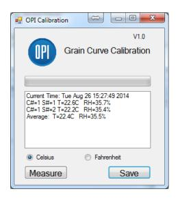
c. The window will show the time of the reading for each of the two sensors and the average for both T and RH. Press the Save button to Save and take note of these readings. The data will be stored in the file C:\Program Files(86)\OPI-Grain Curve Calibration\DS\_Temp.dat
