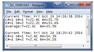
d. To validate the accuracy of the selected curve at cold temperature, place the sealed box in the refrigerator (about 36°F/3°C) for a minimum of 4 hours. Once these steps are complete, plug the OPI USB adapter into your computer and use the OPI Grain Curve Calibration software to measure and save the cold T and RH readings as before.
